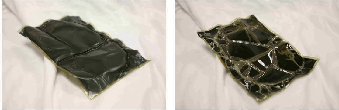
(a) The emulsion side of a deteriorated negative. (b) The acetate side of the same negative. (Courtesy: S. Bailey)
