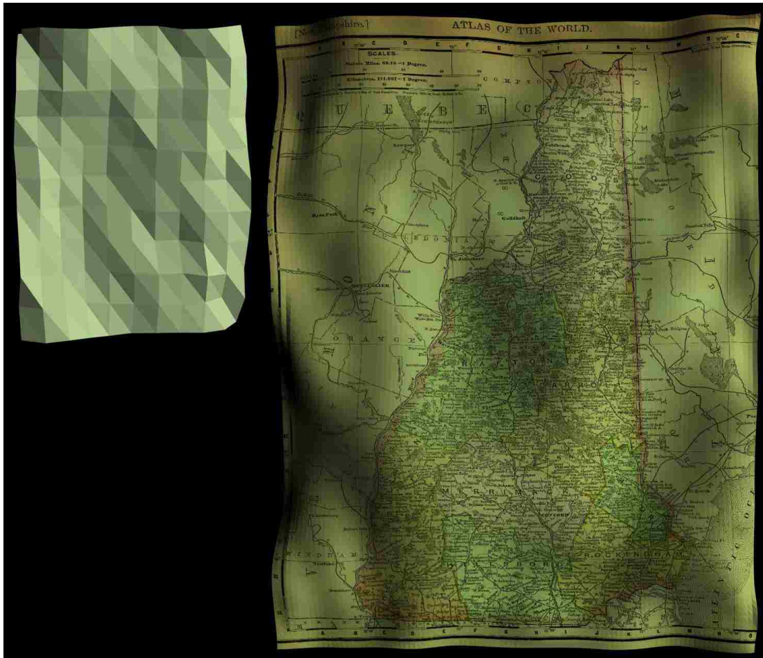
Figure 3.1: The synthetic input image of a distorted map document and paper light probe.
