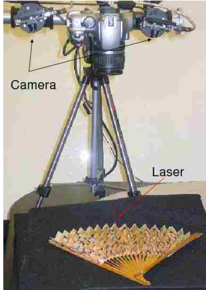
Figure 4.1: A structured-light scanner used for document acquisition.
